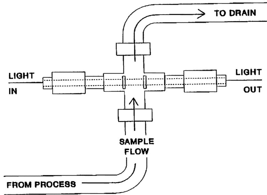
Figure 7. Flow Through Cell
