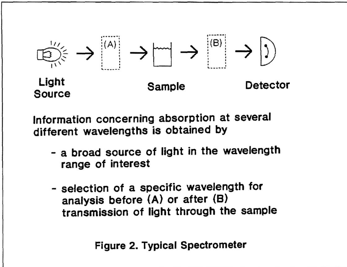
**Figure 2. Typical Spectrometer**
