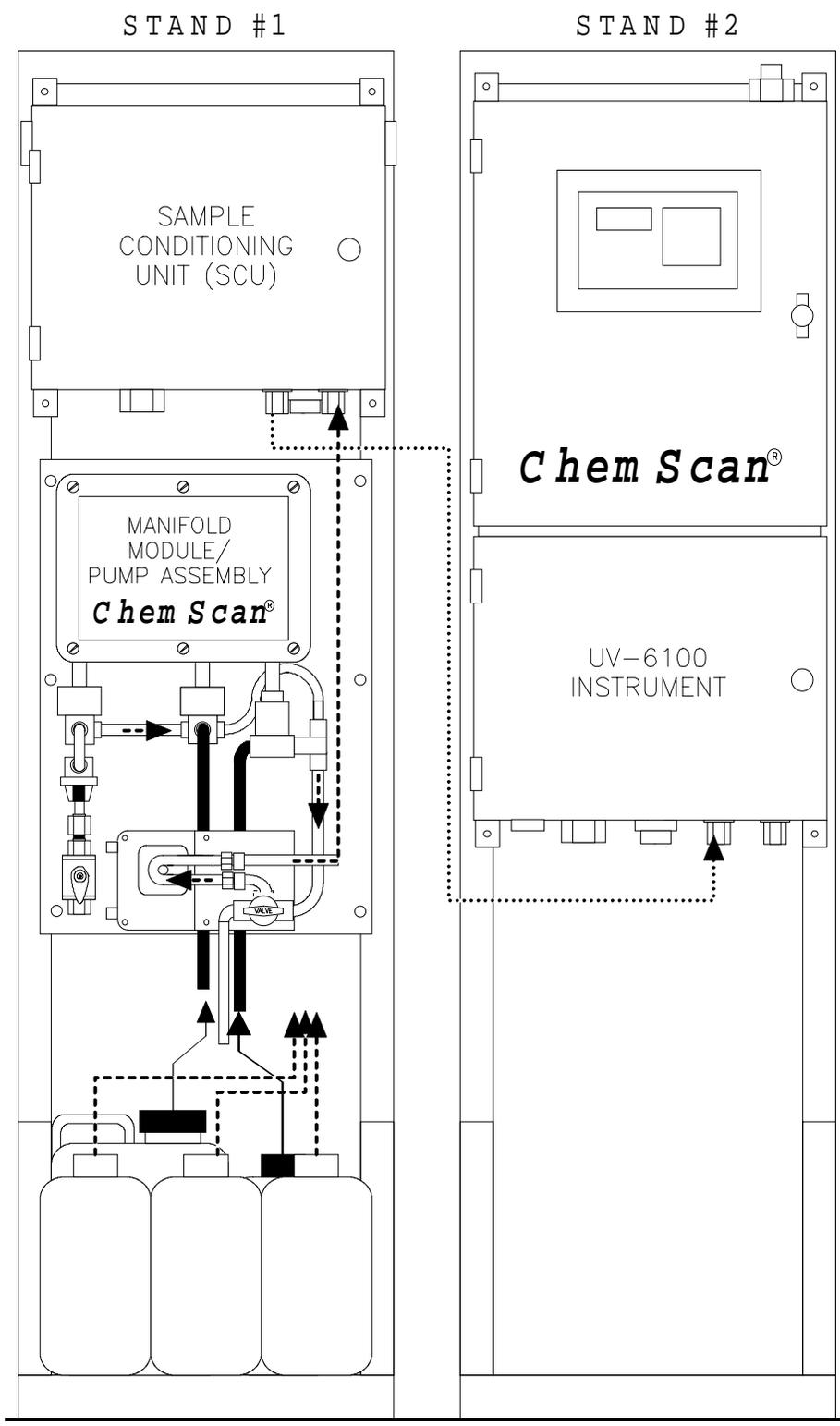
**Figure 1: ChemScan Analyzer System**
