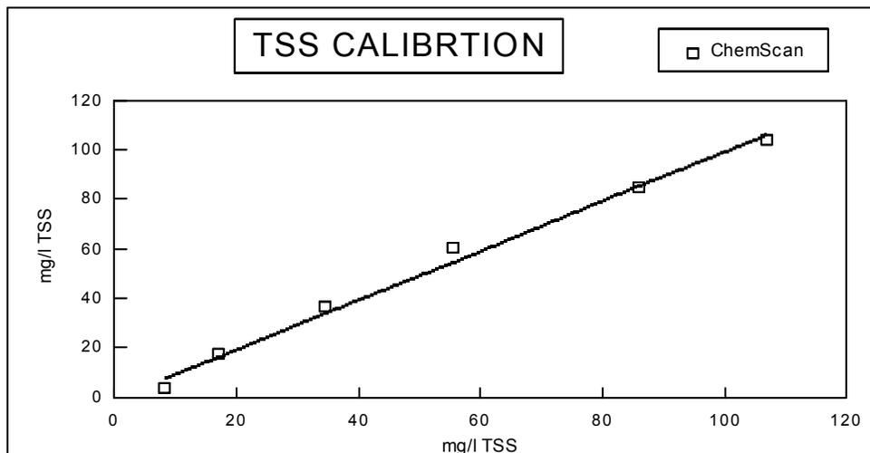
Figure 7: TSS Calibration Curve
